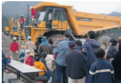
Opportunity to ride a HD605 dump truck HD605: Payload 63,000 kg, flywheel horsepower 533 kW (725 PS)
